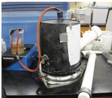
Bench-scale biodigesters are made from PVC pipe, 5-gallon paint buckets, 5-liter water bottles, balloons and hoses.
